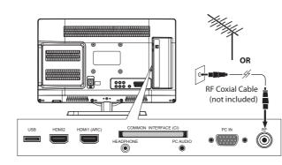
Connect one end of the RE coaxial cable to the aerial socket on the wall and the other end of the cable to the RF (75 $\Omega$ ) socket at the rear right side of your TV.
